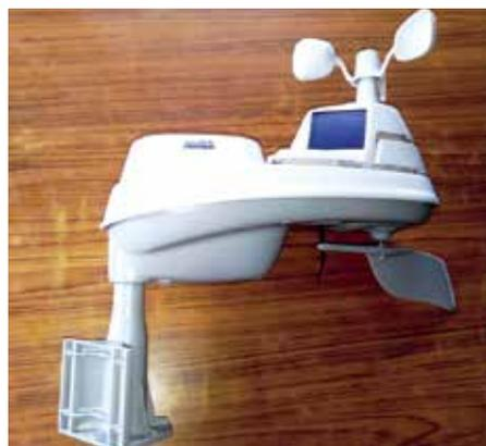
Figure 7: Micro Weather Station Device
